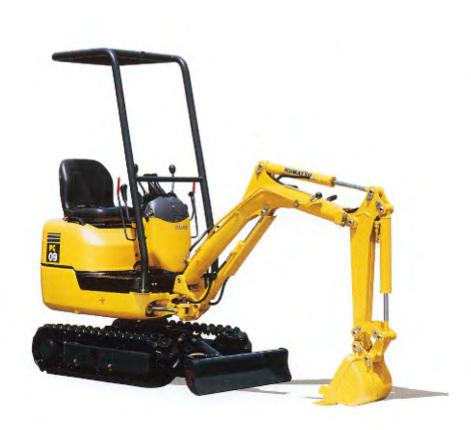
Expandable undercarriage can pass through narrow doorways due to narrow width and undercarriage can be expanded for good stability during excavation.
