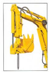
Easily converts from bucket to hydraulic breaker configuration since breaker is stored inside arm when not in use.
